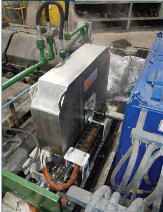
On-line one-strand EDDYeyes industrial unit.
