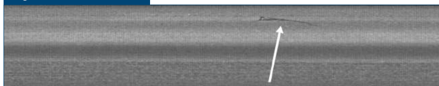
A typical roller crack defect.
