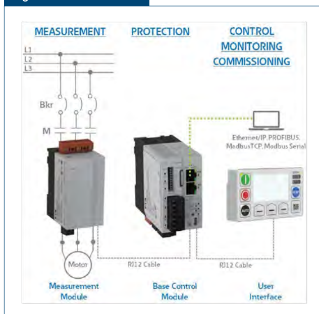
Typical microprocessor-based motor management relay.
